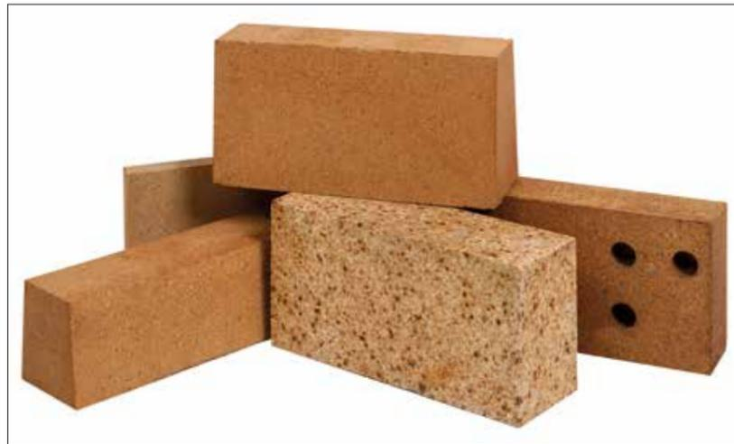
Ultra Fire Bricks are available in a variety of low iron and alkali contents. The high Alumina range utilises various minerals to give 60% and 80% Alumina materials, for the highest Alumina contents tabular and fused Alumina is used.
