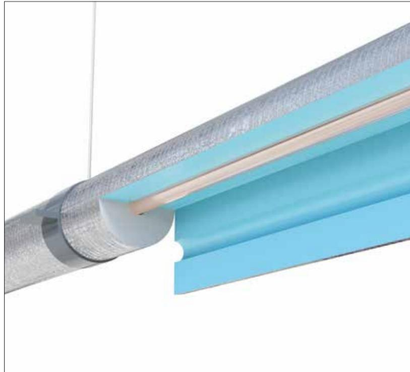
The integral lap aids a fast and efficient installation - simply snap the pipe section around the pipe, remove the backing tape and press into place for a completely sealed joint.
